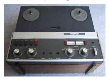
Half track 7.5ips and 15ips with optional Dolby noise reduction. Suitable for location analogue recording. This machine has been optimised for lower noise, lower distortion, and set up to match professional signal levels.
